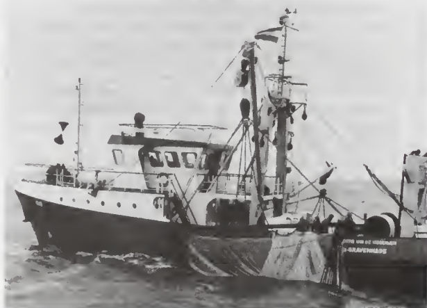
(Left) Dutch outrigger trawler hauling a heavy beam trawl. (Right) Cod being hauled aboard a Russian stern trawler in the Bering Sea.
